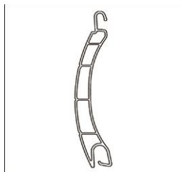
Roller shutter profile K52 with light gaps
